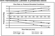
Flow Rate vs. Pressure Data was obtained in vitro using a glycerin/water analog with a viscosity of ≈2.75 cP.
